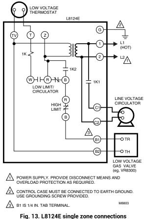
Fig. 13. L8124E single zone connections and internal schematic.
