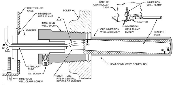
M BEND THE CAPILLARY TUBE TO HOLD THE SENSING BULB IN GOOD THERMAL CONTACT WITH THE IMMERSION WELL AT POINTS (A) AND (B).
