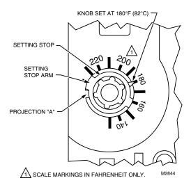
Fig. 22. Setting stop in position to limit the high limit setting to 200°F (93°C).
