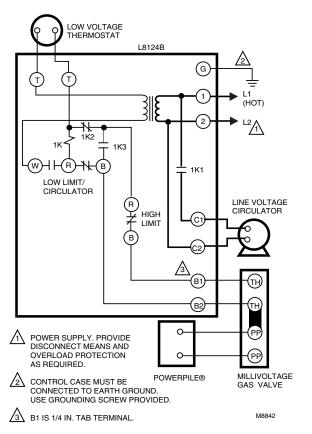
Fig. 11. L8124B single zone connections and internal schematic.
