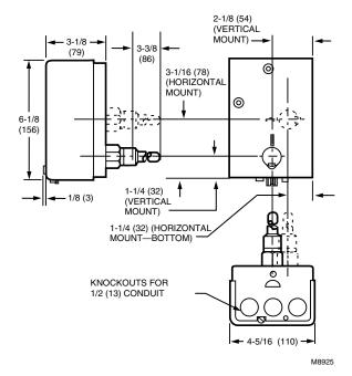
Fig. 1. L8124 mounting dimensions in in. (mm).
