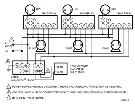
Fig. 15. L8124E in a 24V, gas-fired forced hot water, tankless, zoned pump system.
