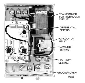
Fig. 5. Internal view of L8124E.
