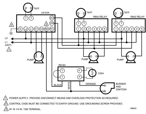
Fig. 10. L8124A in an oil-fired, forced hot water, tankless, zoned, pump system.
