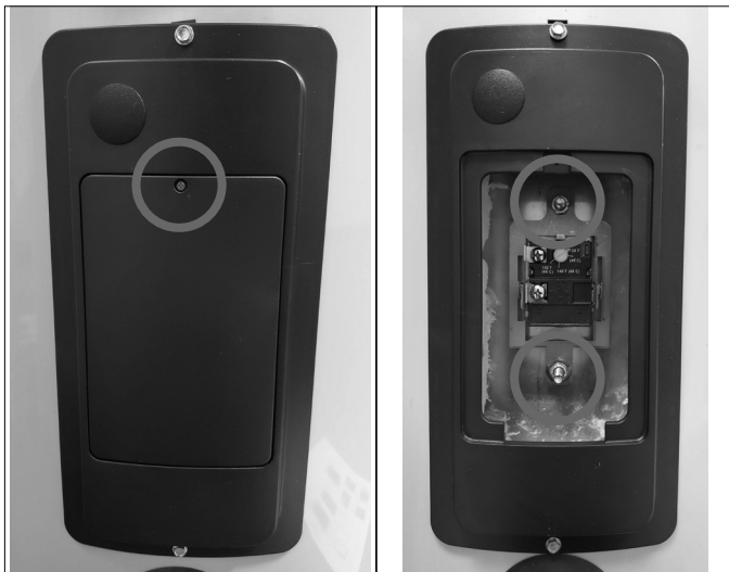
Figure 17 - Screw Securing the Cover
