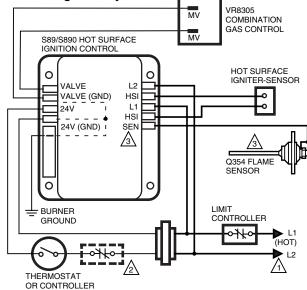
POWER SUPPLY. PROVIDE DISCONNECT MEANS AND OVERLOAD PROTECTION AS REQUIRED. MAKE SURE L1 AND L2 ARE NOT REVERSED; THIS WOULD PREVENT FLAME DETECTION.
