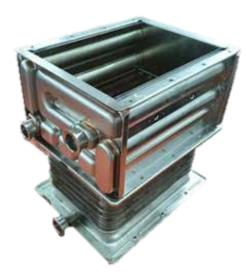
Stainless steel heat exchanger utilizes a unique oval pipe design in the primary heat exchanger to maximize heat transfer for quick hot water, less scale build-up, increased thermal efficiency, and lower maintenance.
