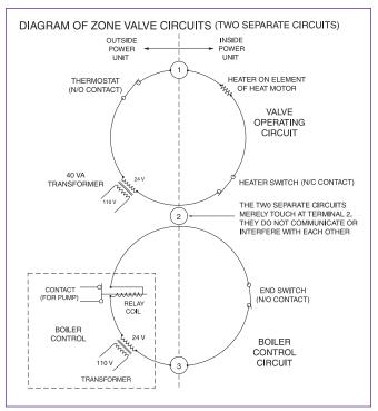
Figure B: Zone Valve Circuits.
