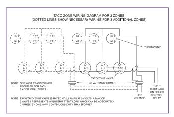
Figure C: Wiring Additional Zones
