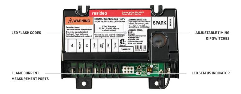
Suitable for use with or without vent dampers the S8610U provides the ignition sequence, flame monitoring and 100 percent safety shutoff for intermittent pilot central furnaces and heating appliances. Enhancements that improve the performance and simplify troubleshooting highlight the latest release of the Universal control.
