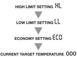
The display will return to boiler temperature (default) if Test/Settings Button in not pressed for 5 seconds.
