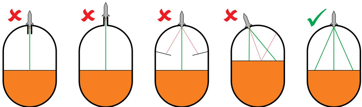
Do not insert a tube, or any other sharp or rough edge inside, or on top of tank.
