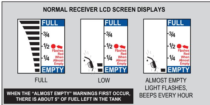
NOTE: DIP switch No. 1 is used for enabling (ON)(factory setting) or disabling (OFF) the audible low fuel level warning. See **Figure 3** on previous page.
