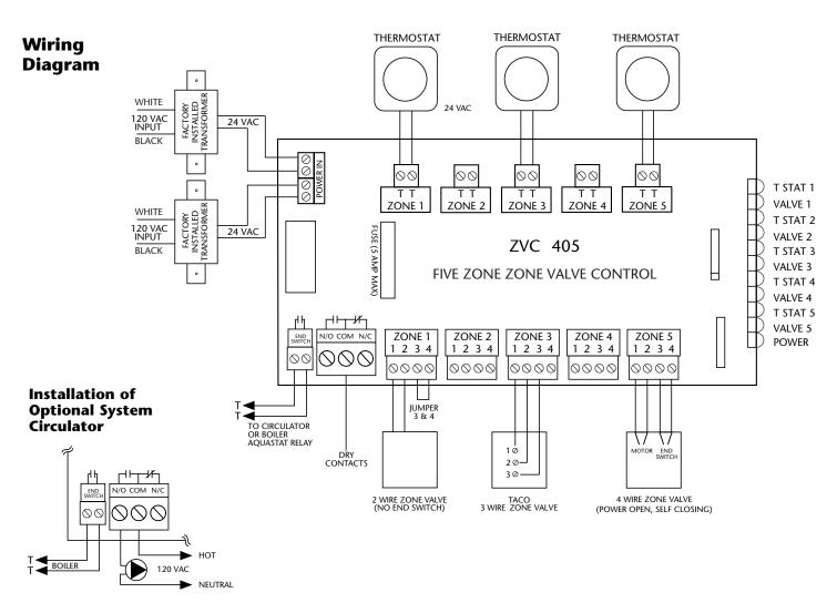
**Operation/External Diagnostics:** When any thermostat calls for heat, the appropriate zone valve is energized and the yellow light goes on. When the zone valve is fully open, the red light goes on and energizes the end switch relay. The green light should always be on, indicating that power is connected.
