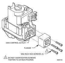
Fig. 1. Fasten Flange to Valve with 25 in.- lbs (2.8 N·m) Torque.
