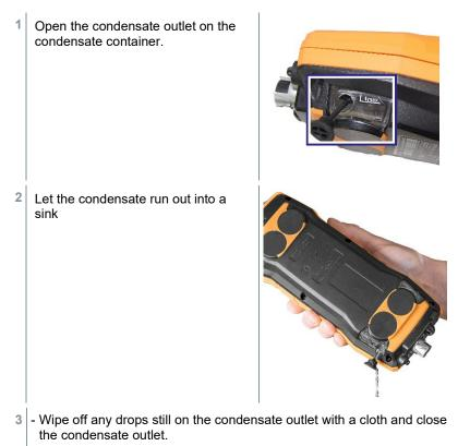
The condensate outlet must be completely closed, otherwise incorrect measurements could occur due to infiltration of external air.
