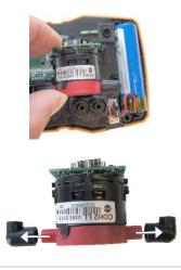
For NO sensor: Remove auxiliary circuit board.
