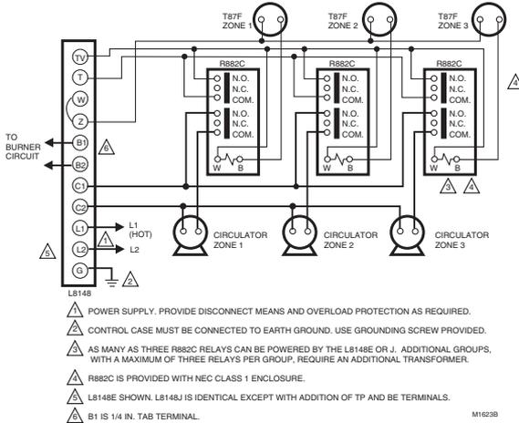
Fig. 10. Multizone system with R882C switched circulator.
