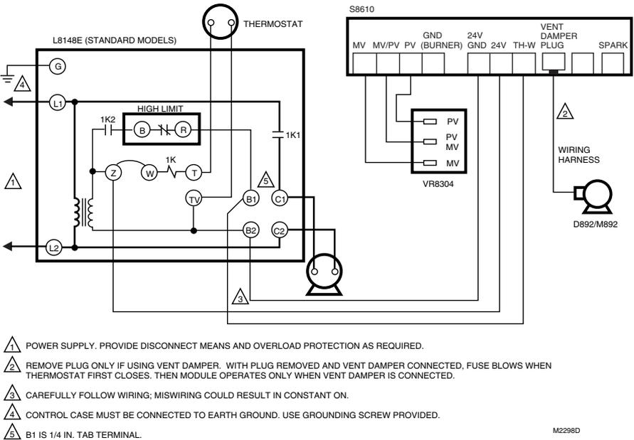
Fig. 8. Wiring L8148E with S8610 automatic vent damper plug and vent damper.
