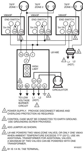
Fig. 6. Wiring L8148E with multizone valves.
