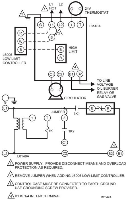
Fig. 2. External connections and internal schematic for L8148A.
