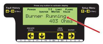
Last Fault Alert – Real diagnostics that spell out what the problem is when your technician arrives on the job even if control has been reset. Below is a snapshot of what you could see on a no heat call.
